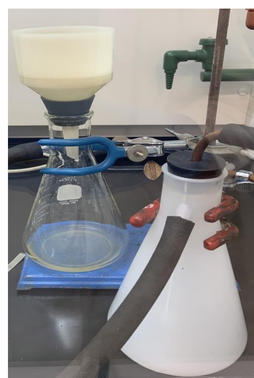
Figure 1. Vacuum filtration system for drying algae.
