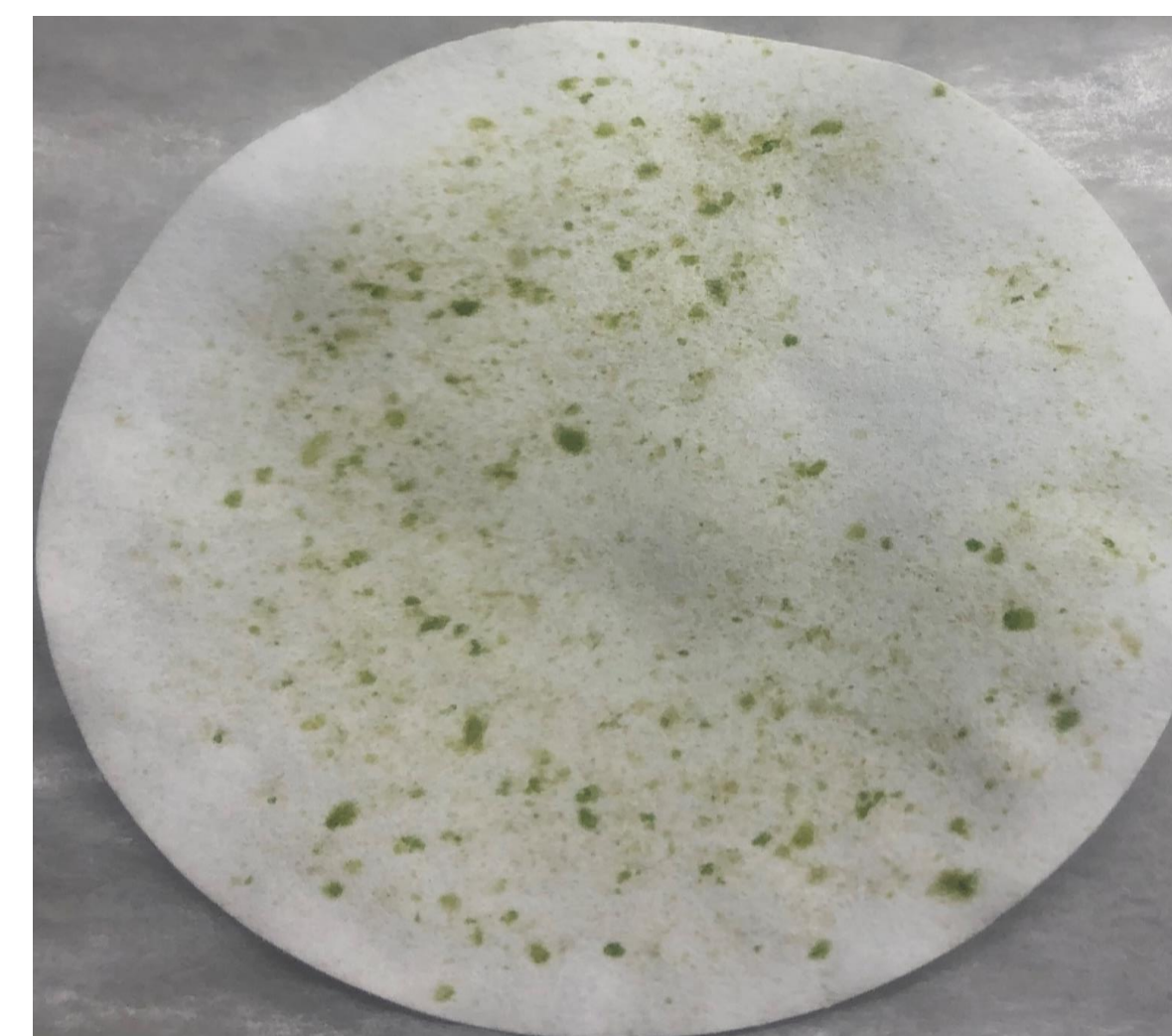
Figure 6. Run 4: Vacuum filtrated algae dried in a tray dryer.
