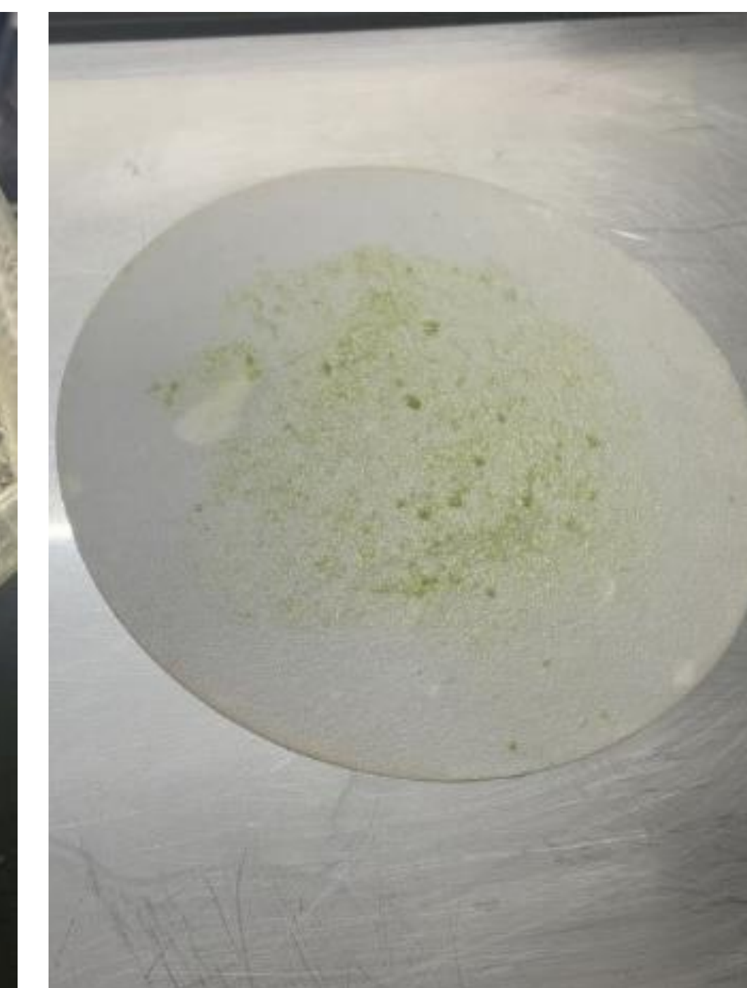
Figure 4. Run 2: Algae after gravity filtration dried using a tray dryer on filter paper.
