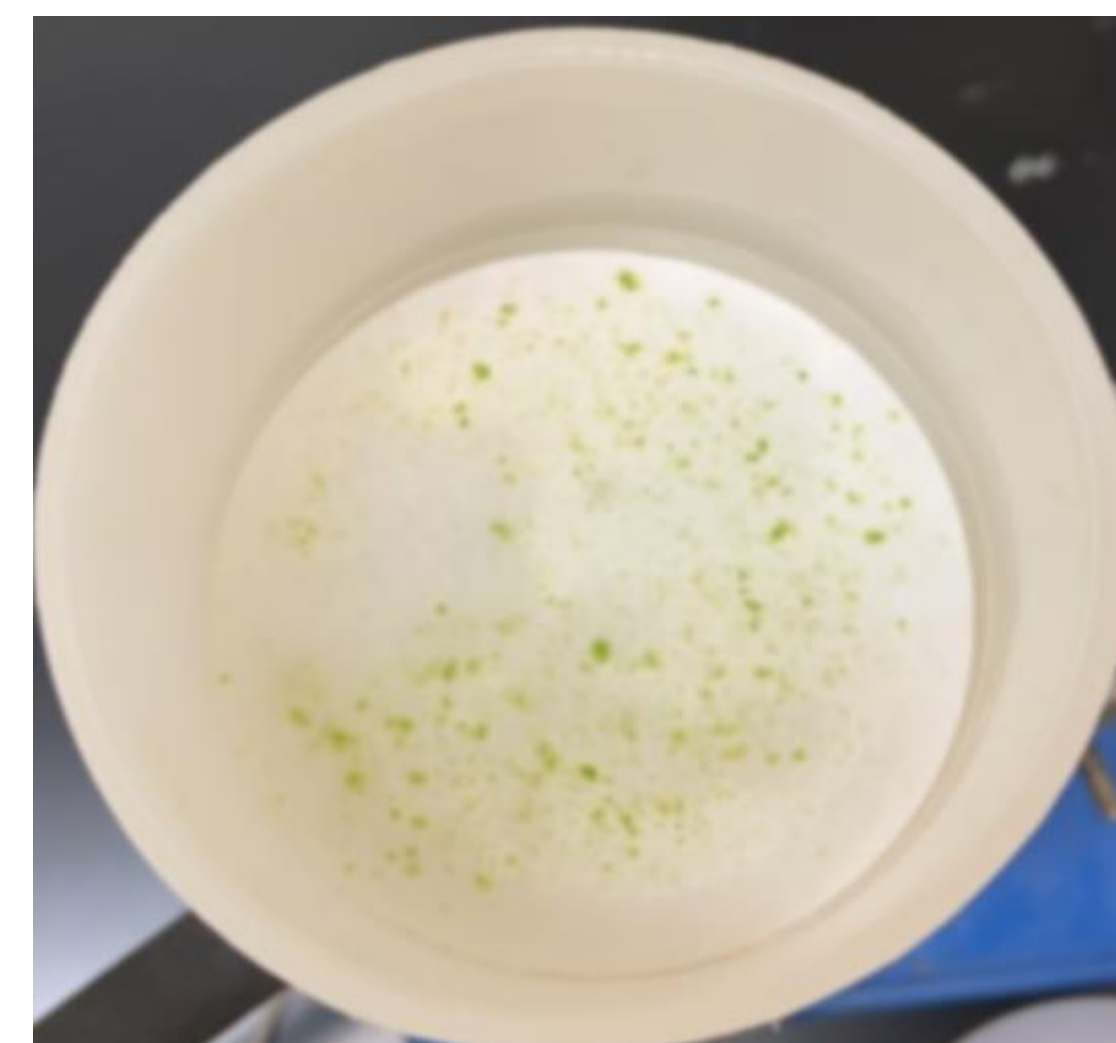
Figure 5. Run 3: Algae dried on filter paper using vacuum filtration.
