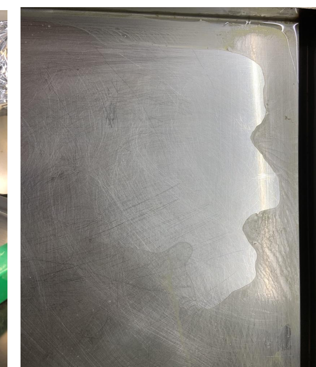
Figure 10. Run 6: Partially dried algae after three hours in a tray dryer
