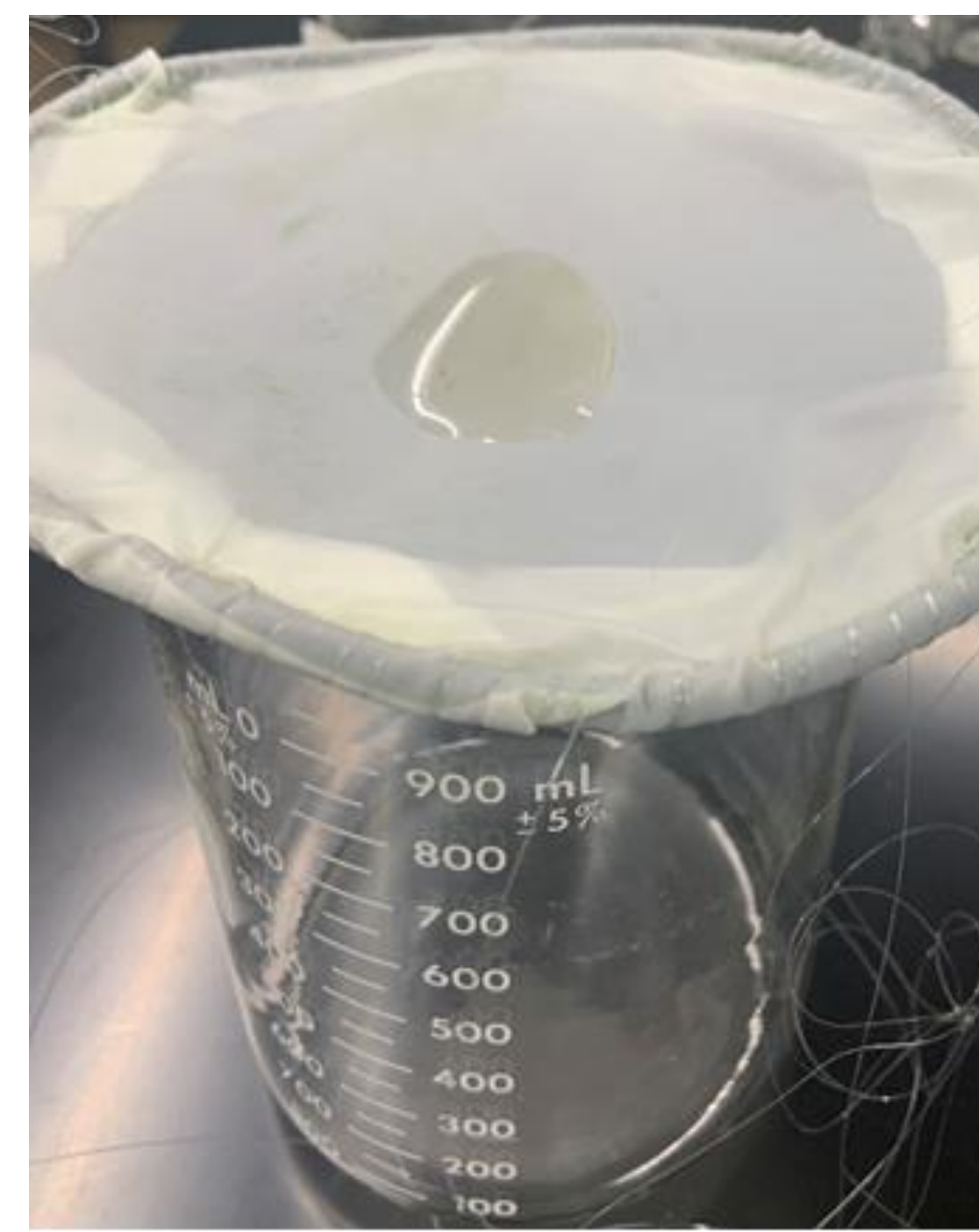
Figure 2. Run 1: Algae gravity filtered through a 20µm mesh fabric.
