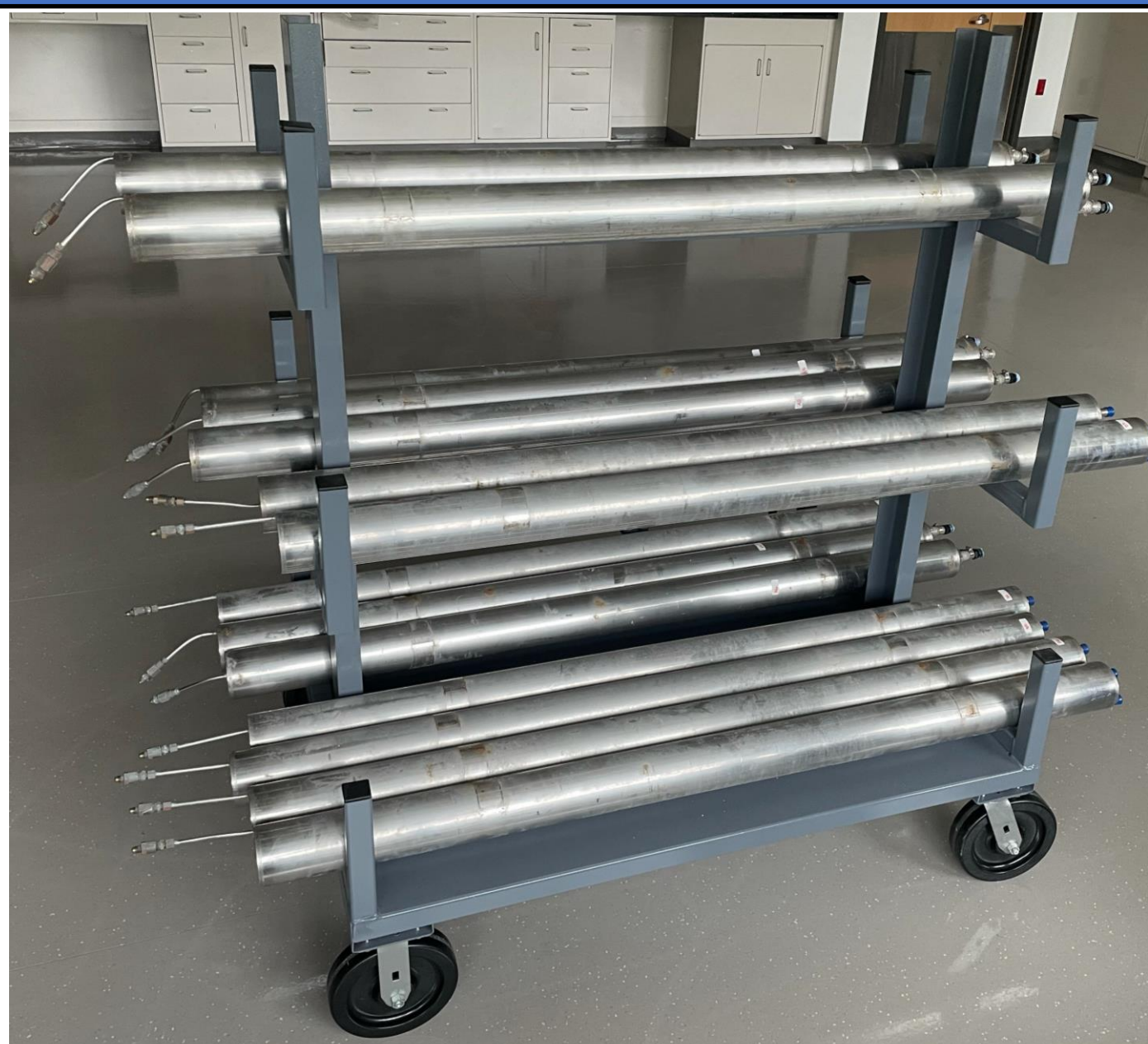
Hydrogen storage system
